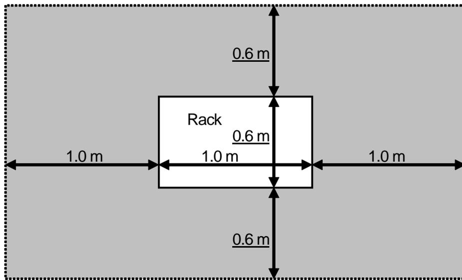
Figure 5.1.1 Standalone Installation
