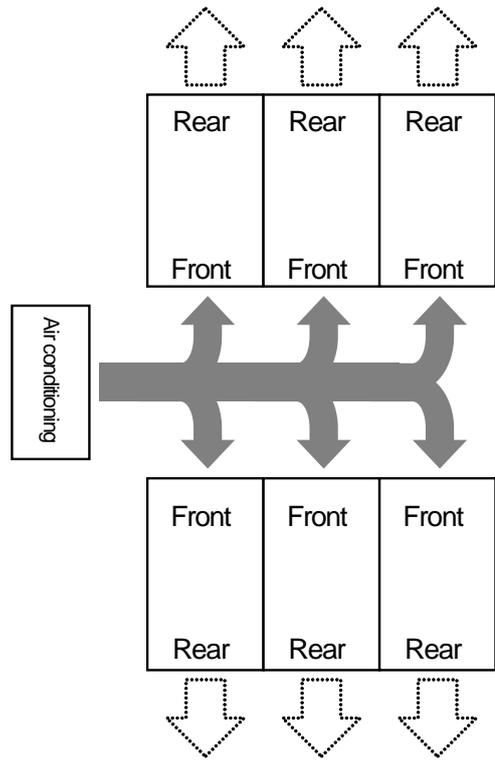
Figure 5.4 Air Flow (When Multiple Racks are installed)
