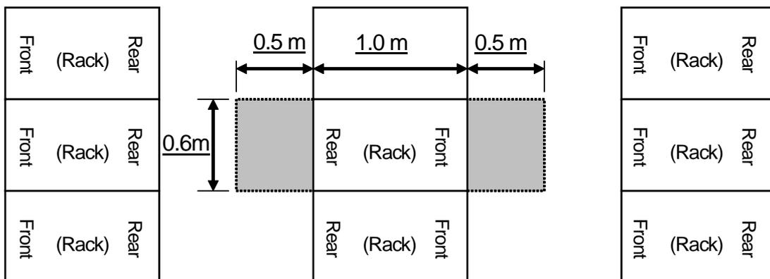
Figure 5.1.2 Coupled Installation
