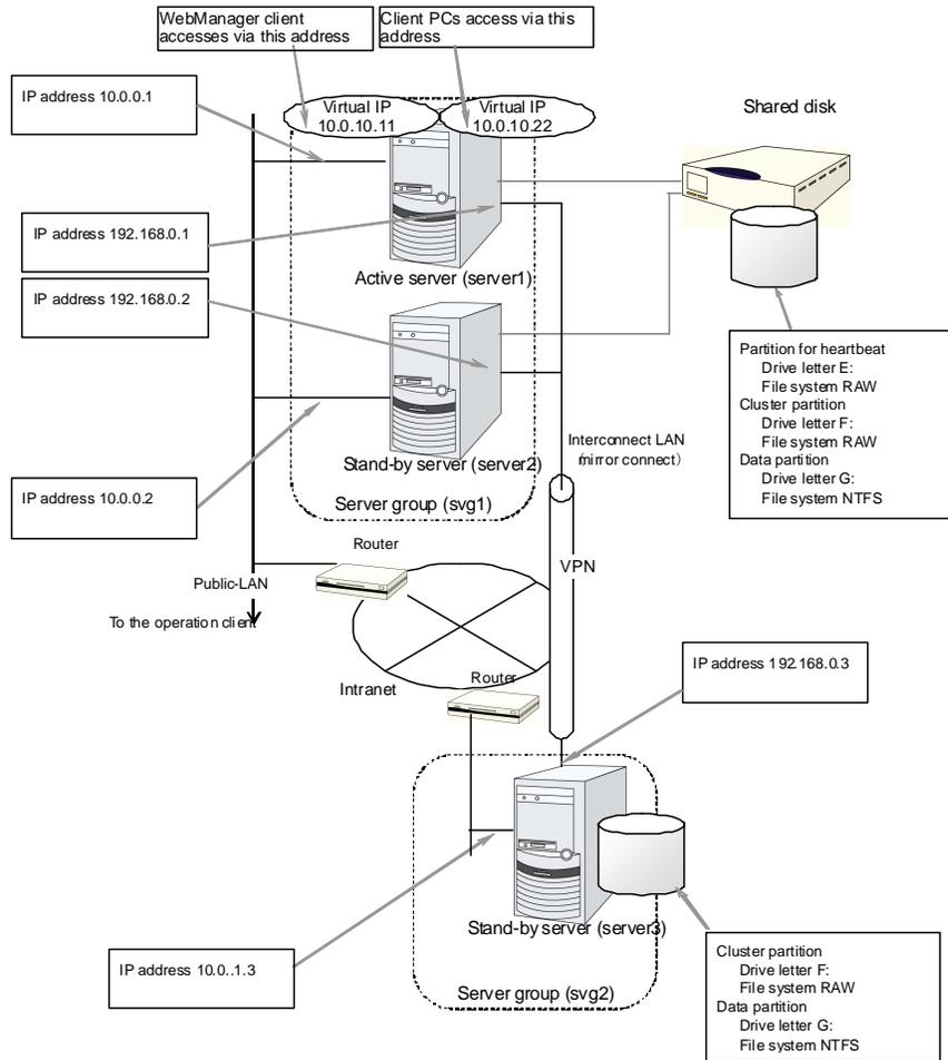
**Figure 2-7: Sample of the remote cluster environment when the hybrid disk is used**
