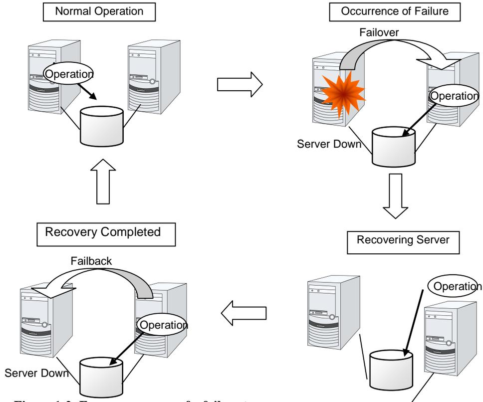
Figure 1-2: From occurrence of a failure to recovery
