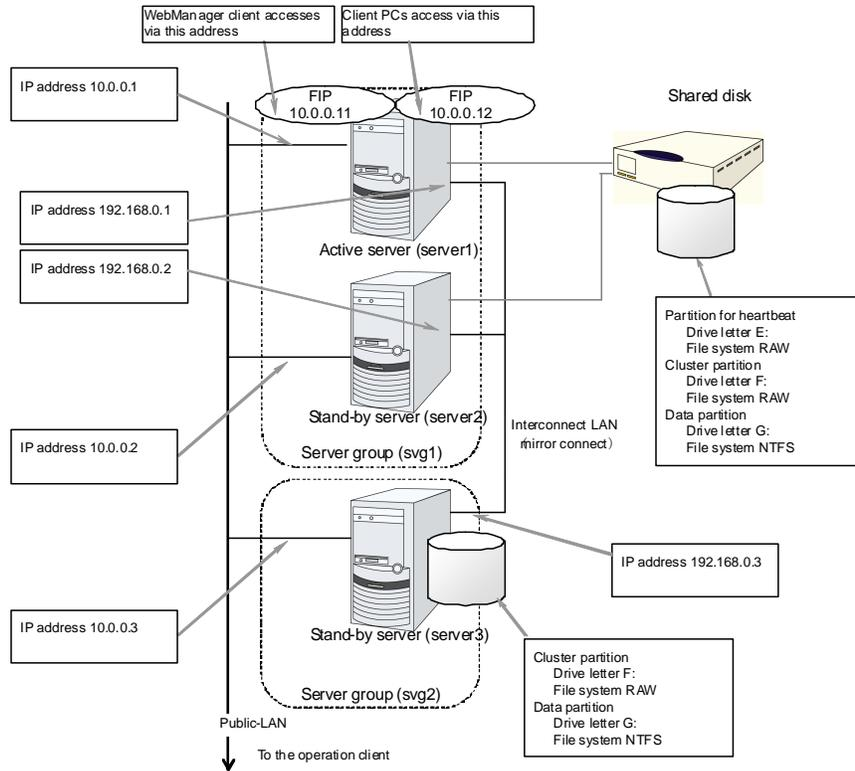
**Figure 2-6: Sample of the hybrid disk type cluster environment when**
