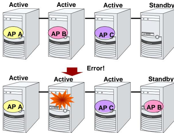
Figure 1-9: N Server to M Operation configuration
