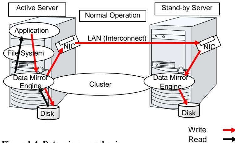
**Figure 1-4: Data mirror mechanism**
