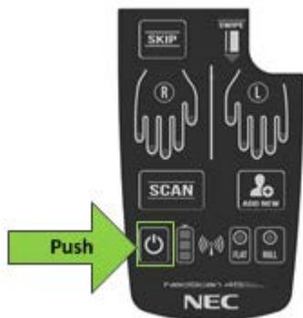
Figure 13: Shutting Down NeoScan 45
