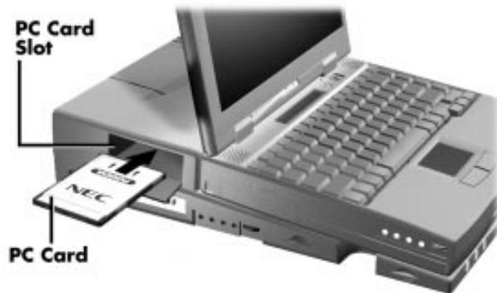
*Inserting a PC card in the MiniDock*
