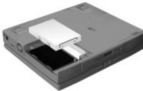
*Inserting the hard disk drive*
