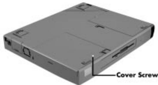
*Replacing the screw that secures the cover*
