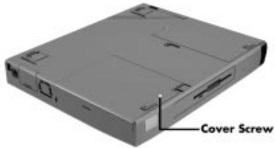
*Removing the screw that secures the cover*
