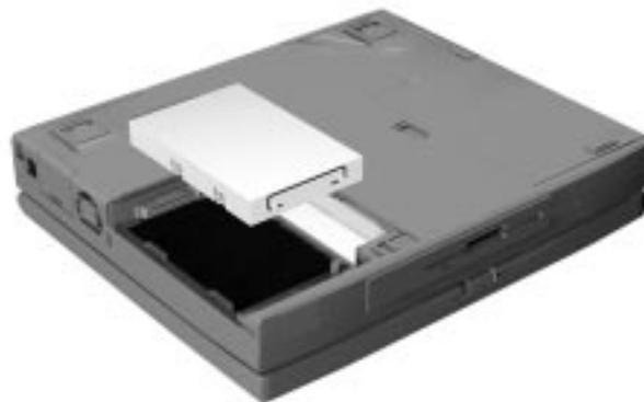
*Inserting the hard disk drive*
