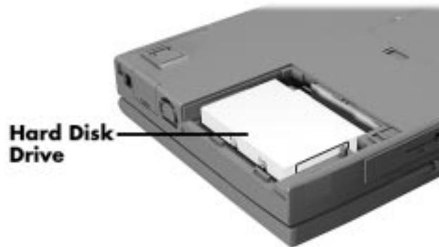
*Removing the hard disk drive*
