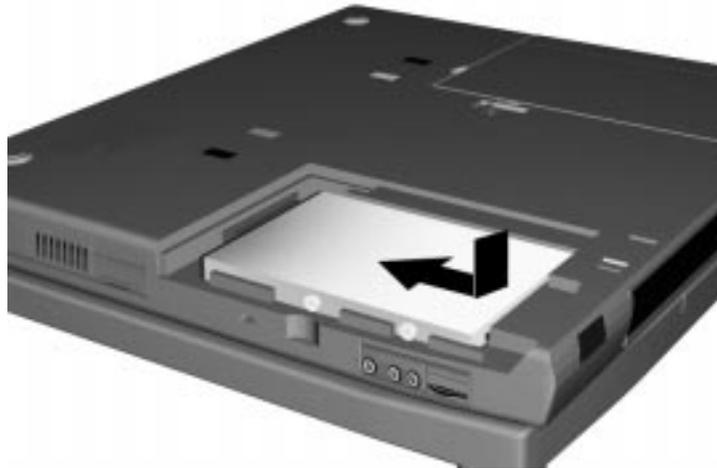
*Inserting the hard drive*
