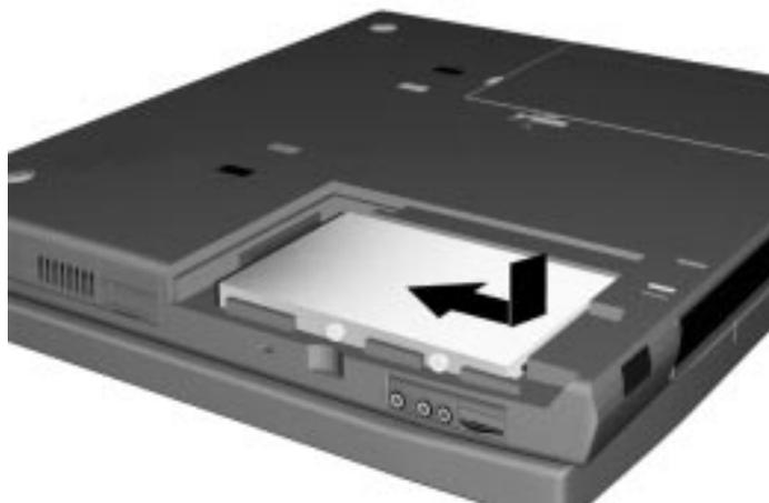
*Inserting the hard disk drive*
