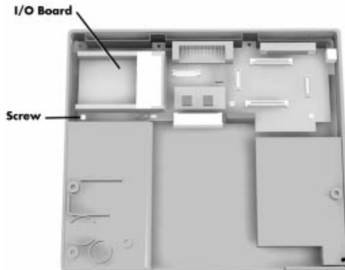
**Figure 4-15** Removing the I/O Board
