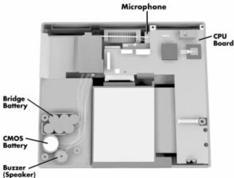
**Figure 4-13** Removing the CPU Board
