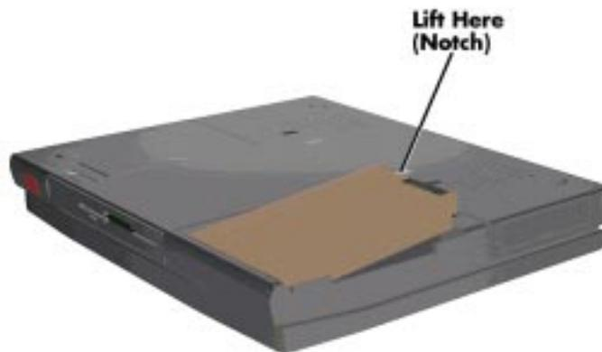
**Figure 2-6** Removing the Battery
