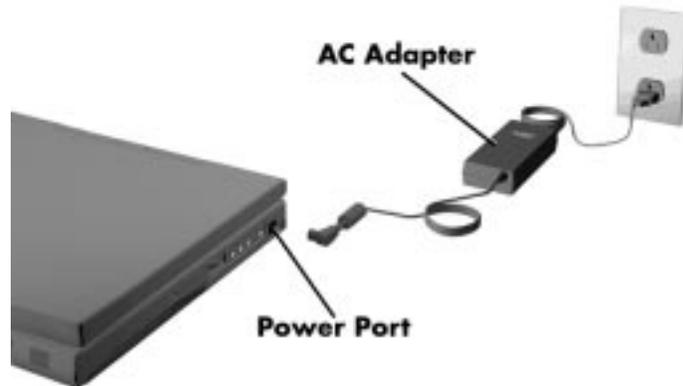
**Figure 2-1** *Connecting the AC Adapter*
