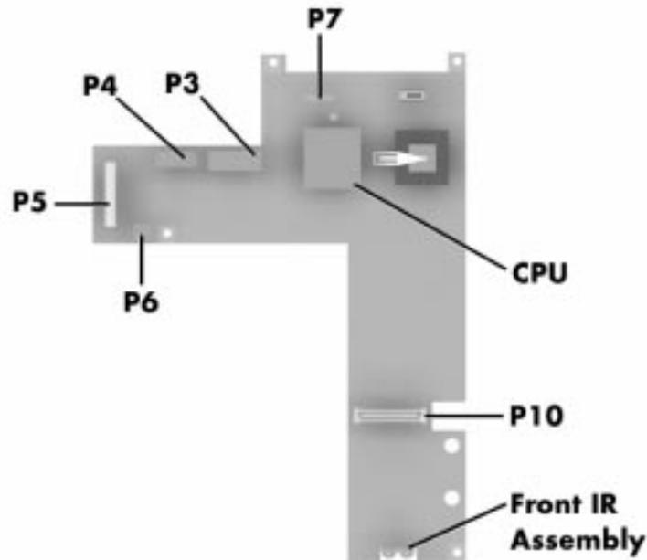
*Figure 1-12 CPU Board Layout*
