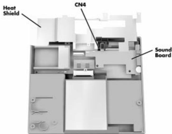
**Figure 4-14 Heat Shield, Sound Board**
