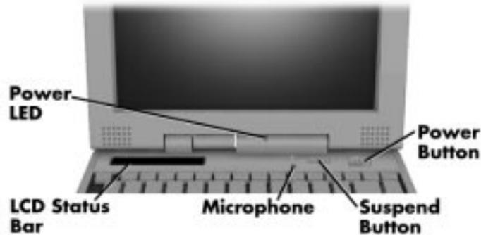
**Figure 2-10 Keyboard Panel LEDs and Controls**
