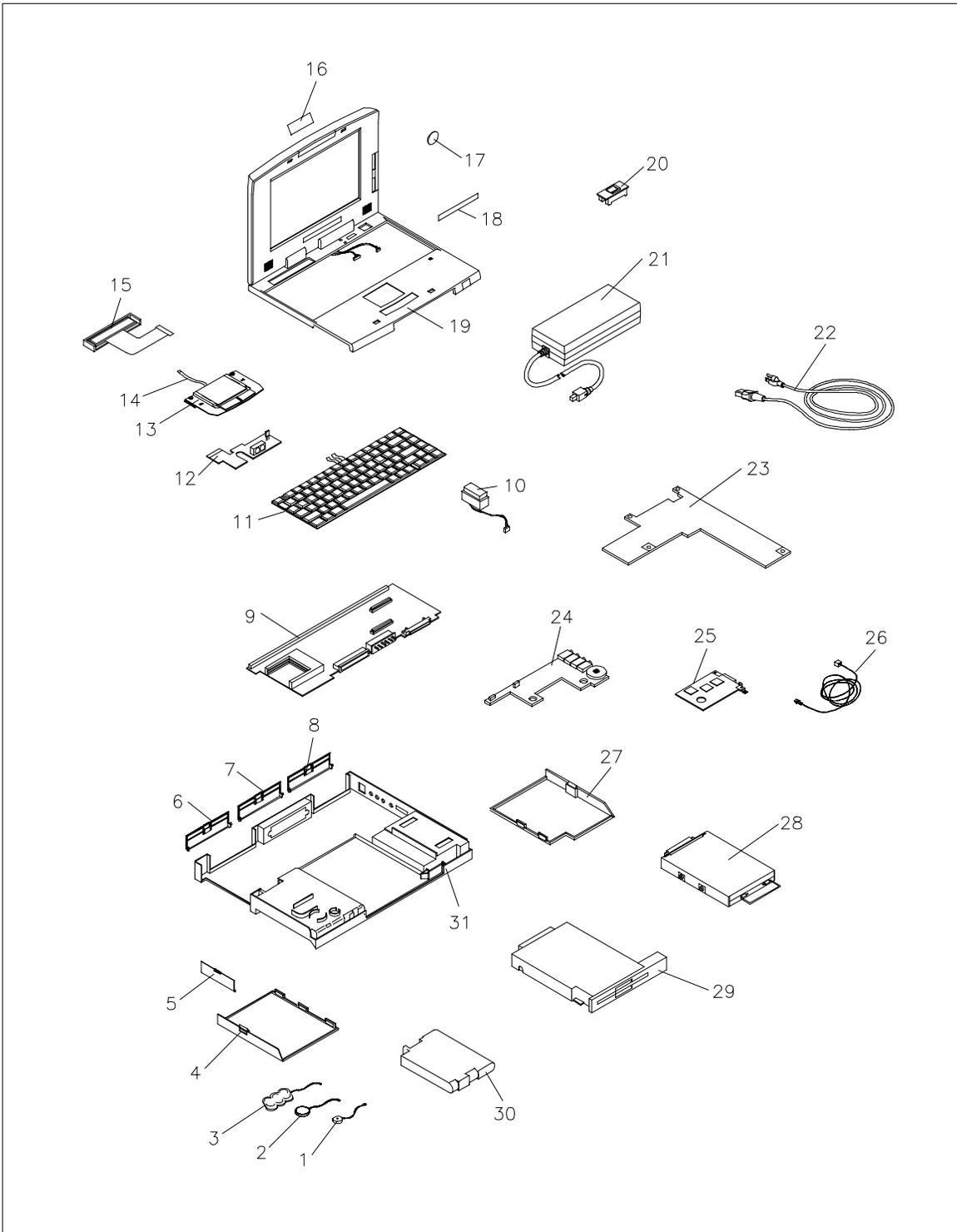
**Figure 4-16 NEC Versa Models 6050MH (PC-6240-91803) & 6050MX (PC-6240-A1803) Illustrated Parts Breakdown**
