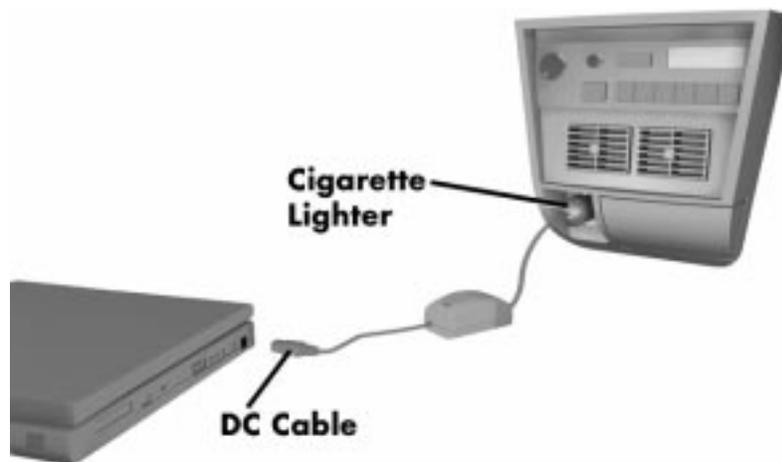
**Figure 2-9** Connecting the Car DC Adapter
