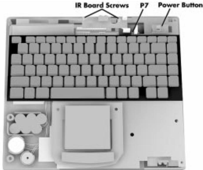
**Figure 4-9** Removing the Power Button, Rear IR Assembly, Keyboard
