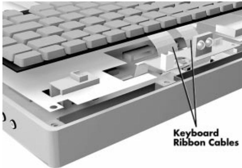
*Figure 4-10 Disconnecting Keyboard Cables*
