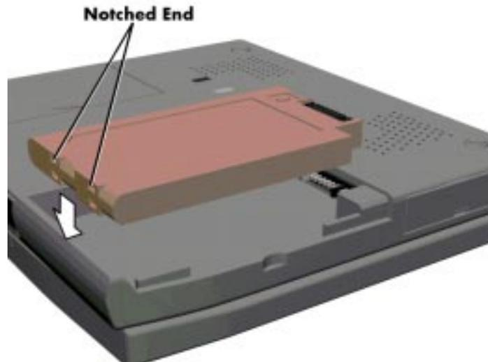
**Figure 2-7** *Inserting the Battery Pack*
