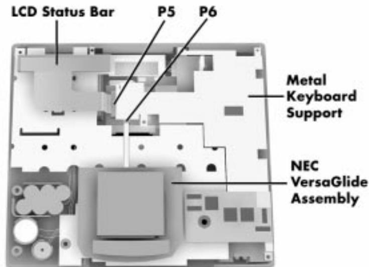
**Figure 4-11** LCD Status Bar, VersaGlide Assembly, Modem Board, Metal Keyboard Supports
