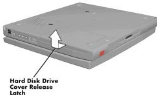
**Figure 4-1** Removing the Drive Bay Cover
