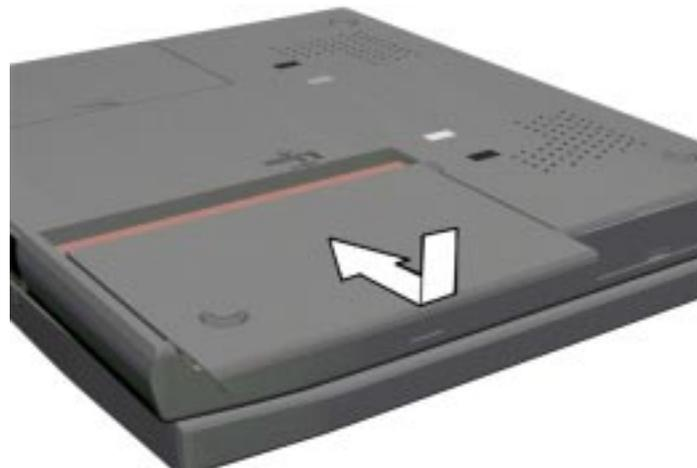
**Figure 2-8** *Replacing the Cover*
