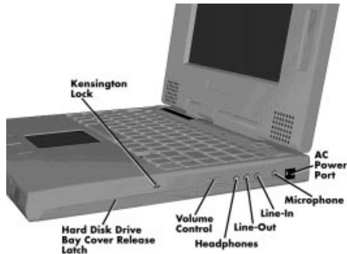
*Figure 2-11 Right Side Panel Controls/Ports*
