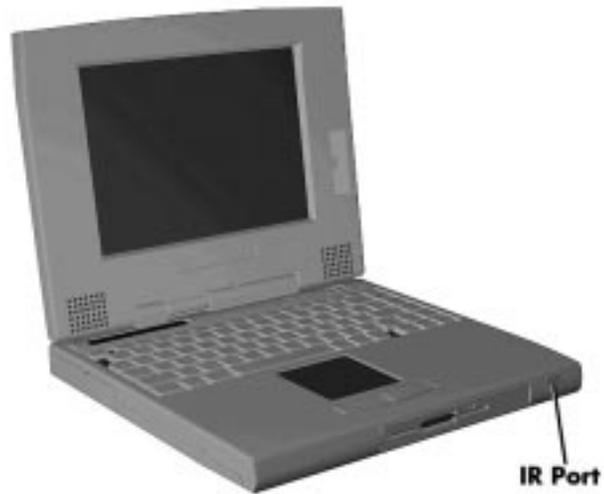
**Figure 1-8 Front IR Assembly Location**
