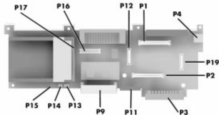
*Figure 1-15 I/O Board layout*
