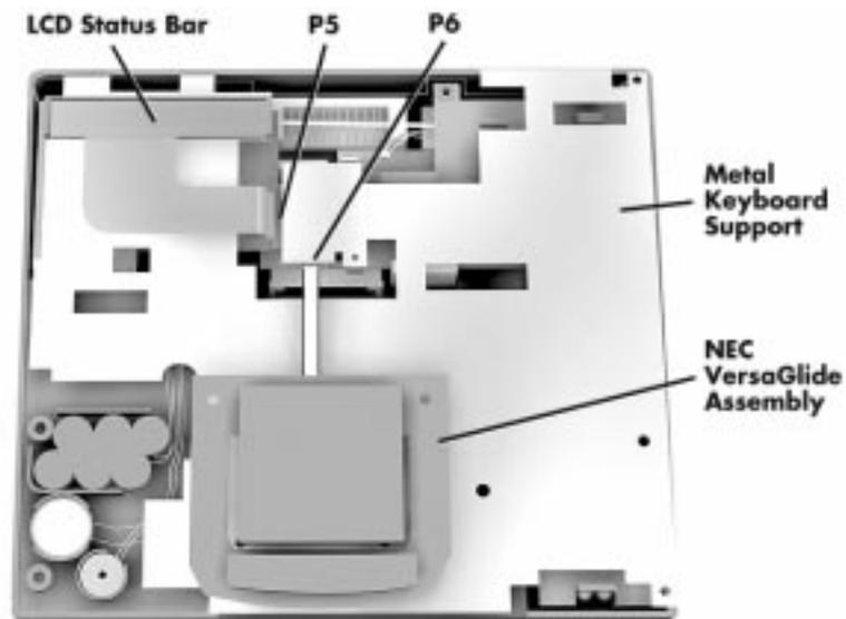
**Figure 4-11** LCD Status Bar, VersaGlide Assembly, Metal Keyboard Support
