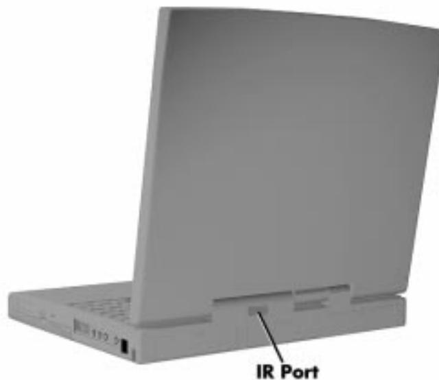
**Figure 1-9 Rear IR Assembly Location**
