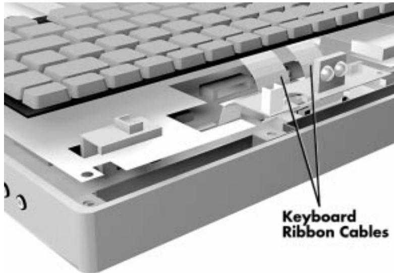
*Figure 4-10 Disconnecting Keyboard Cables*
