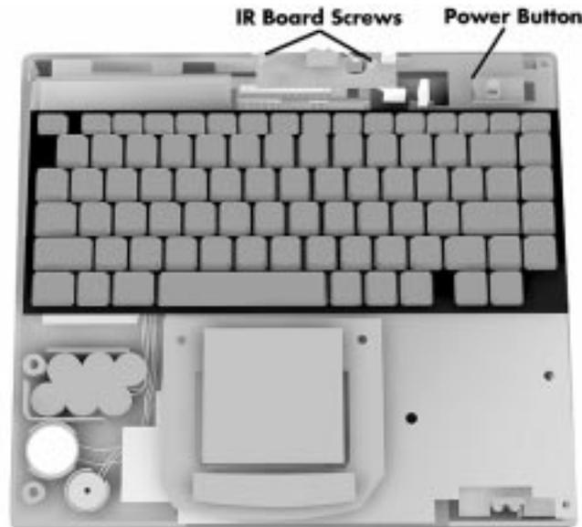
**Figure 4-9** Removing the Power Button, IR Board
