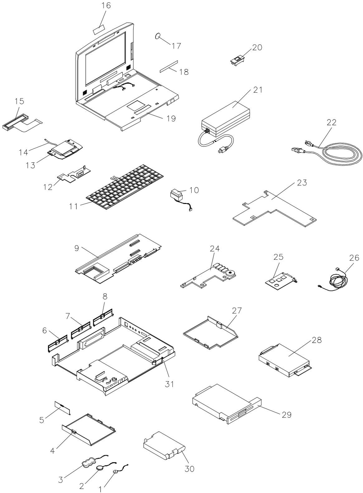
**Figure 4-16 NEC Versa 6000 Illustrated Parts Breakdown**
