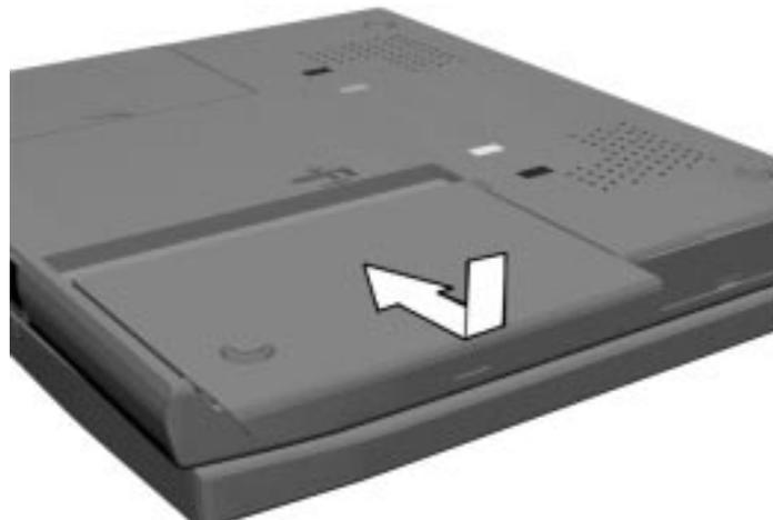
**Figure 2-8** *Replacing the Cover*
