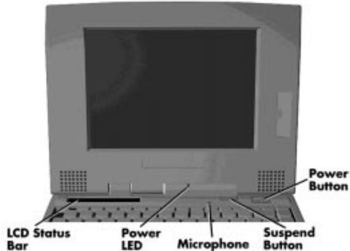
*Figure 2-10 Keyboard Panel LEDs and Controls*
