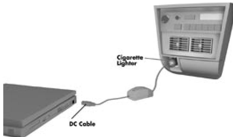
**Figure 2-9** *Connecting the Car DC Adapter*
