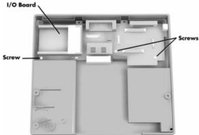
**Figure 4-15** Removing the I/O Board
