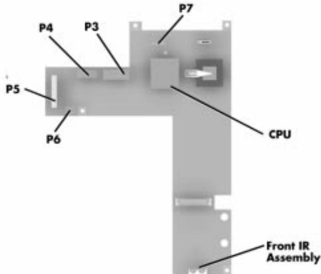
*Figure 1-13 CPU Board Layout*
