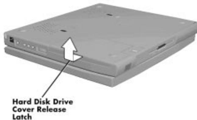
**Figure 4-1** Removing the Drive Bay Cover
