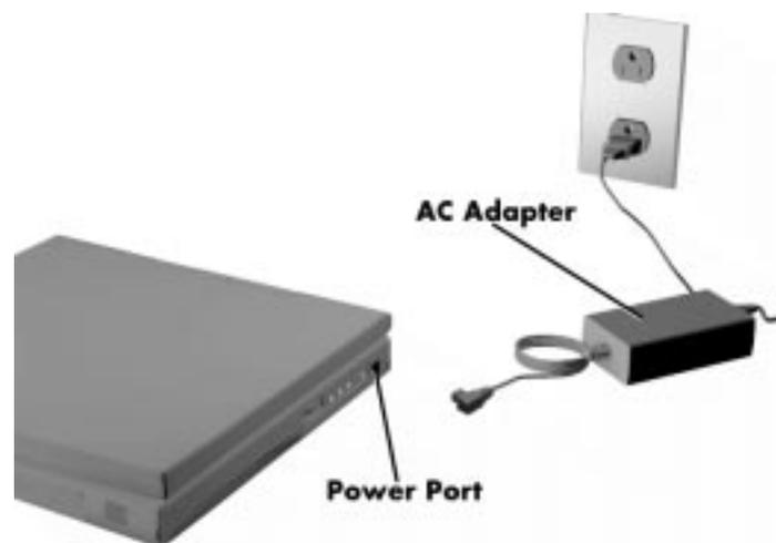
**Figure 2-1** Connecting the AC Adapter
