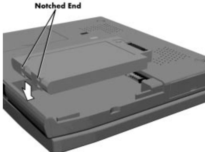
**Figure 2-7** *Inserting the Battery Pack*
