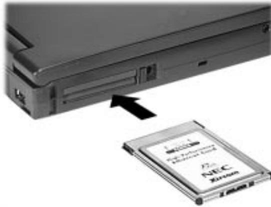
*Inserting a PC card*
