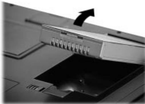
*Removing the battery pack*
