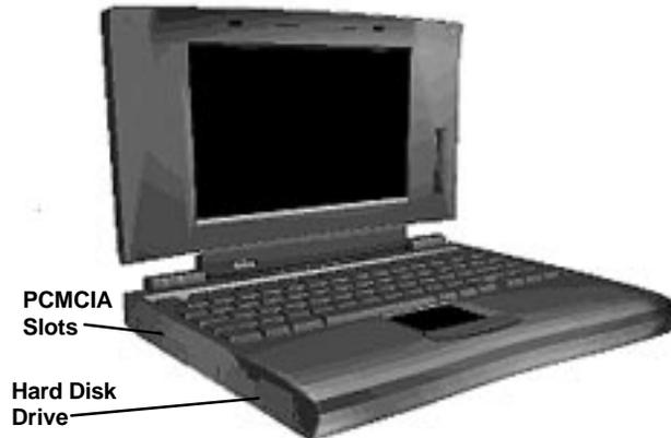
**PCMCIA Slots** — PCMCIA is a standard interface for peripheral devices like fax/modems, local area network (LAN) cards, storage cards, and pagers. A PCMCIA card is about the size and shape of a credit card and inserts into one of the two slots.
