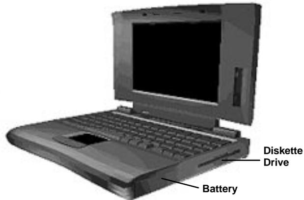
**Diskette Drive** — You can save your files to diskette and install software from diskette using the diskette drive, called drive A.
