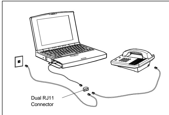
*Dual telephone and modem connection*
