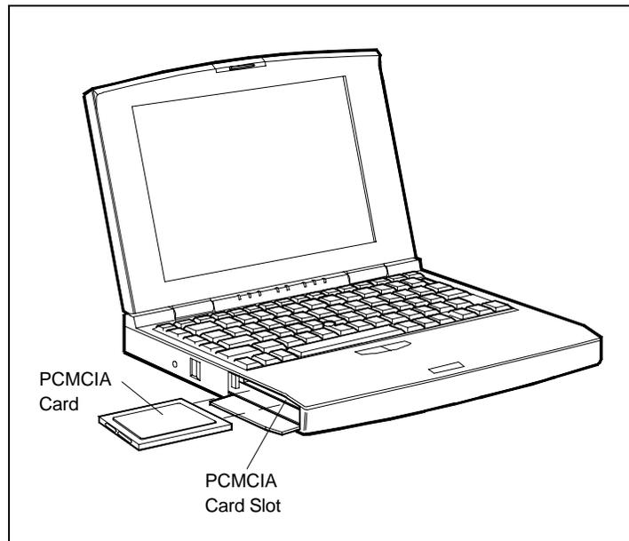
*Installing the modem card*
