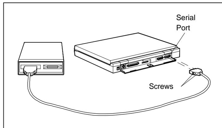
*Attaching a serial device*
