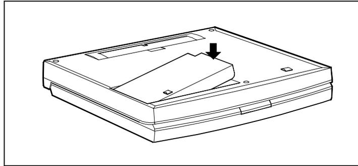
*Inserting the battery pack*
