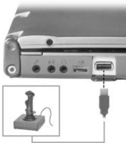
USB devices called USB hubs can serve as connection ports for other USB peripherals. Only one device needs to be plugged into your NEC Versa. Additional peripherals can be connected in a daisy chain configuration where one device is connected to another in a series. Up to 127 devices can be connected together in this way.
