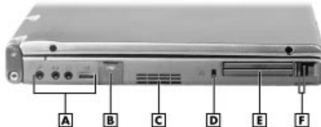
**A** - Audio Ports and Volume Control **B** - USB Port **C** - Fan Vent **D** - Kensington Lock Slot **E** - PC Card Slot **F** - PC Card Ejection Buttons
