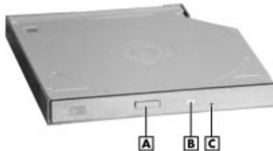
**A** – Release button   **B** – Status LED   **C** – Emergency Eject Hole
