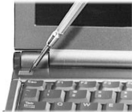
3. Press down using slight pressure on the right hand side of the keyboard retainer and slide to the left.
