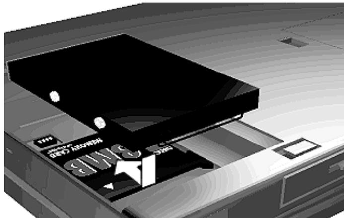
*Inserting the drive*
