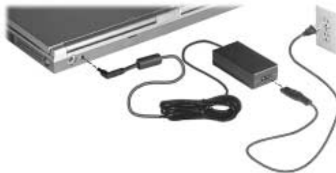
Connecting the AC adapter to an NEC Versa VX or VXi system
