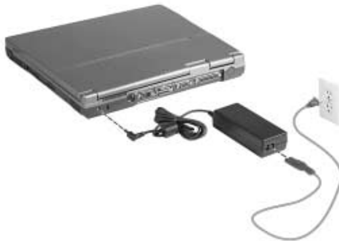
Connecting the AC adapter to an NEC Versa VX or VXi system
