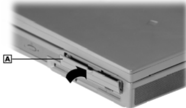
A – Drive Access Panel
