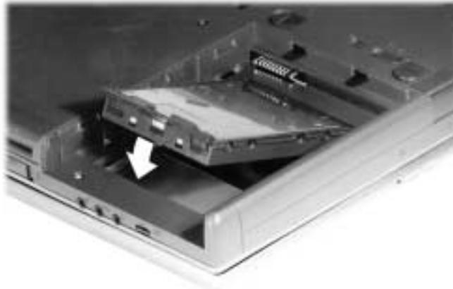
2. Align the drive connector with the connector in the drive bay.
