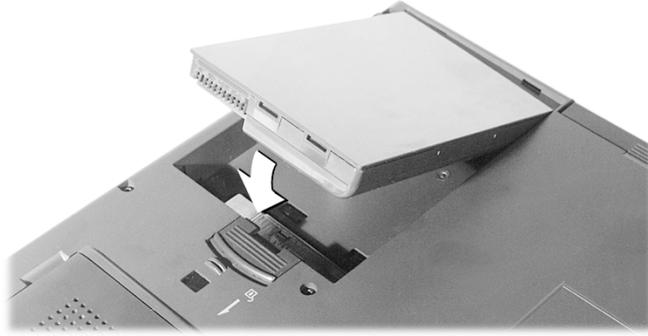
3. Gently place the battery into the battery bay until you hear a click indicating that it is securely locked in place.
