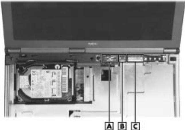
A – Connector P40 (underside)    B – Connector P42    C – Connector P41
