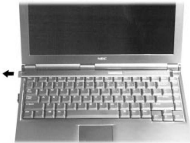
4. Gently lift up the edge of the keyboard nearest the LCD and slide the keyboard toward the LCD screen to release the tabs that secure it.
