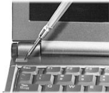
3. Press down using a slight pressure on the right hand side of the keyboard retainer and slide to the left.
