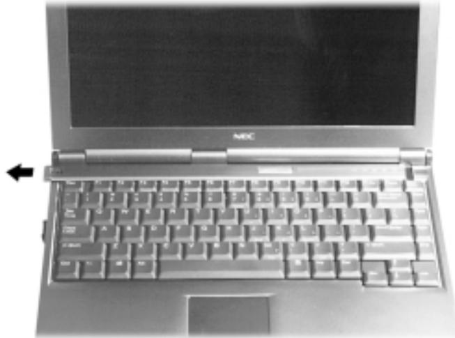
5. Gently lift up the edge of the keyboard nearest the LCD panel and slide the keyboard toward the LCD screen to release the tabs that secure it.
