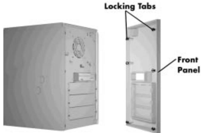
*Removing the front panel*
