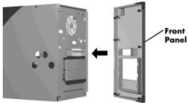
*Aligning the front panel*
