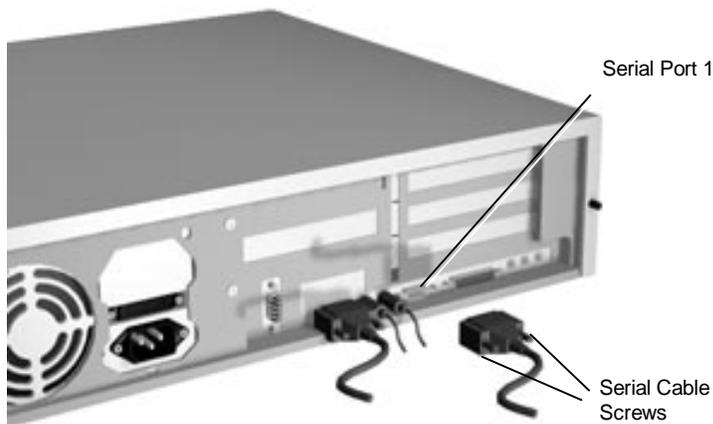
**Figure 3-28** Connecting an RS-232C Cable to the Desktop
