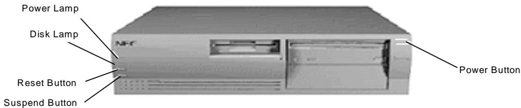
**Figure 2-4 Power Button, Lamps, and Suspend Button**
