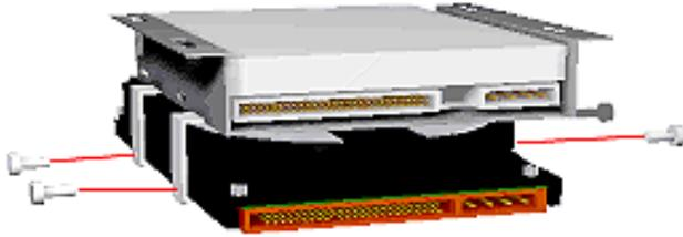
**Figure 3-21 Securing a 3 1/2-Inch Drive**
