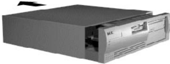
**Figure 5-2 Removing the System Unit Cover**
