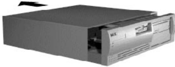
**Figure 3-2 Releasing the Cover**
