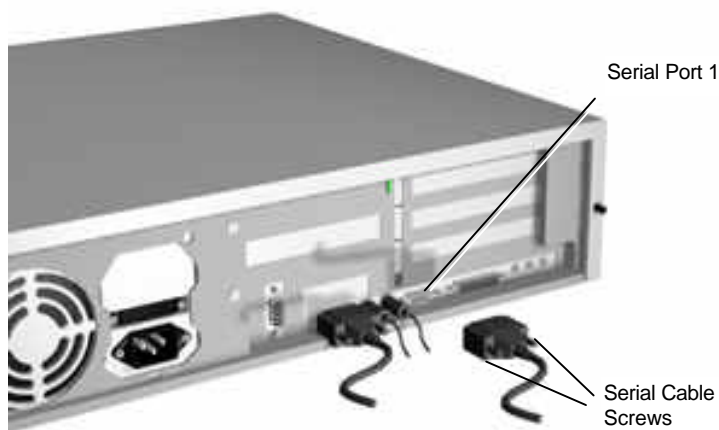
Figure Section 3-43 Connecting an RS-232C Cable to the Desktop
