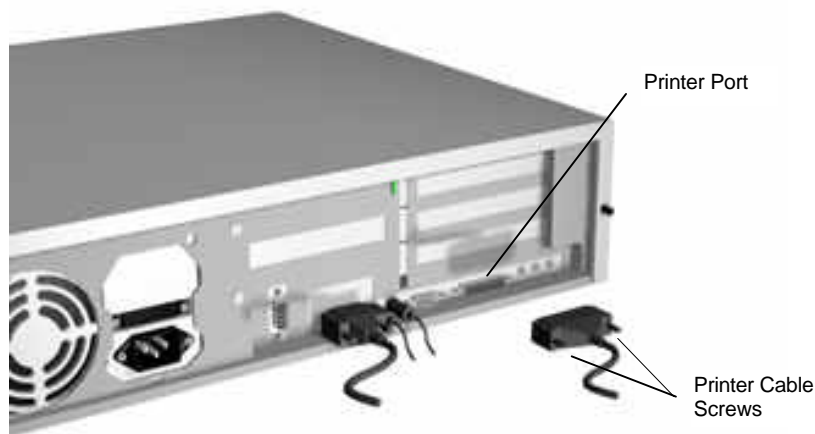
Figure Section 3-41 Connecting a Printer Cable
