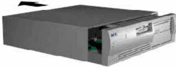
Figure Section 5-2 Removing the System Unit Cover
