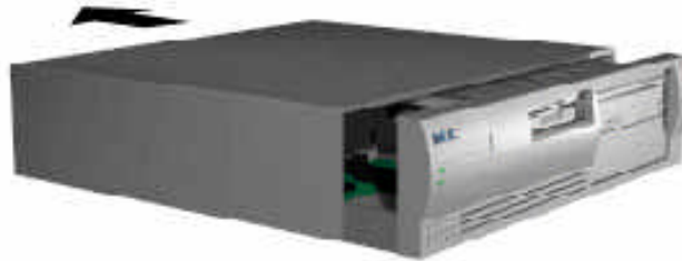
Figure Section 3-2 Releasing the Cover
