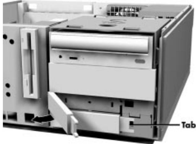
*Removing the blank panel*
