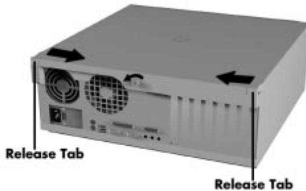
*Loosening the screw and pressing the tabs*
