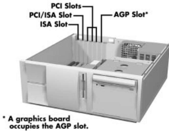
Figure 3-3 Locating Expansion Slots
