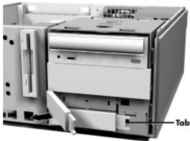
Figure 3-21 Removing the Blank Panel
