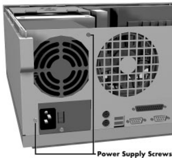
Figure 5-10 Removing the Power Supply Screws
