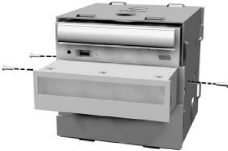
Figure 5-5 Removing the 5 1/4-Inch Device Screws
