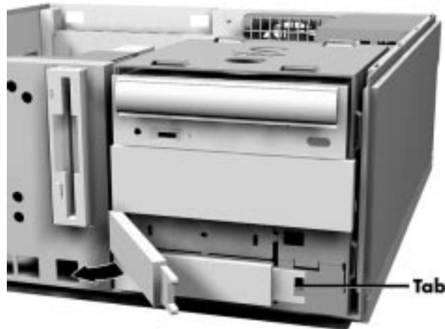
**Figure 3-18** *Removing the Blank Panel*
