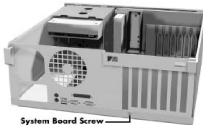
**Figure 5-10** Removing the System Board Screw
