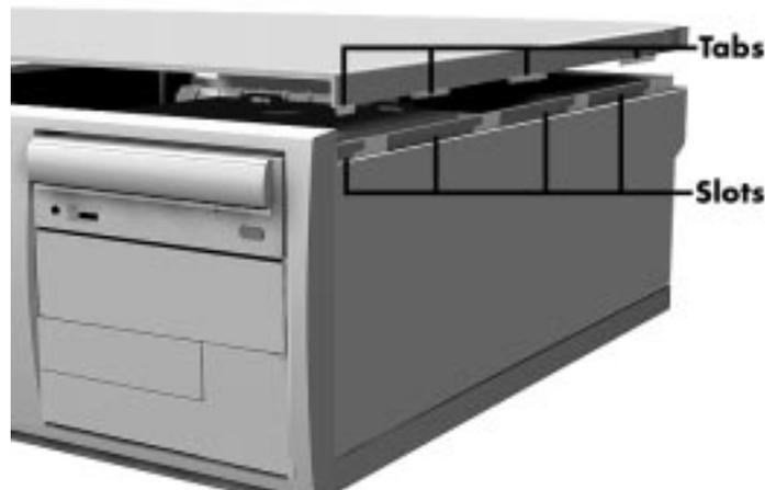
**Figure 3-3** *Aligning the Tabs*
