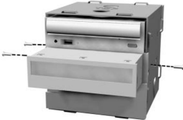
**Figure 5-5** *Removing the 5 1/4-Inch Device Screws*
