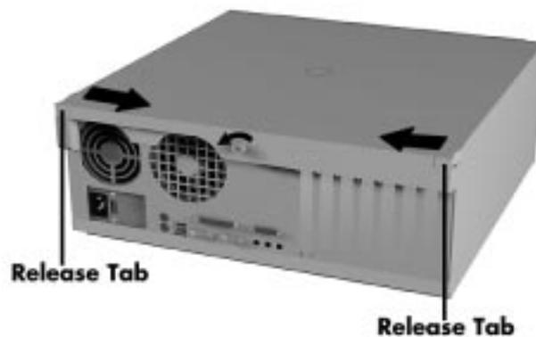
**Figure 3-1** *Loosening the Screw and Pressing the Tabs*
