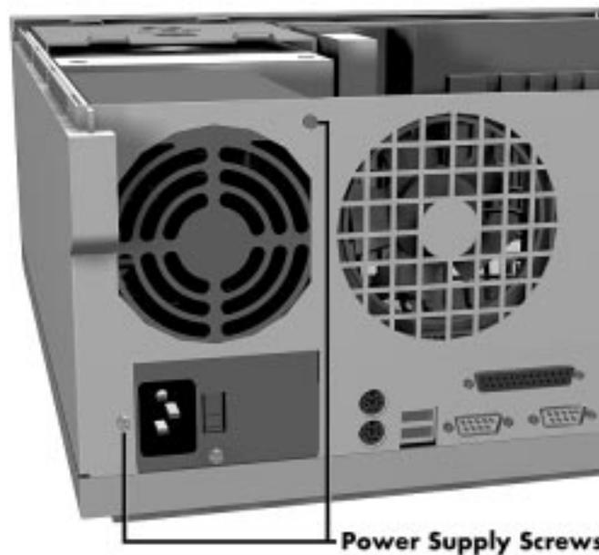
**Figure 5-9** *Removing the Power Supply Screws*
