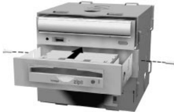
*Installing the device*
