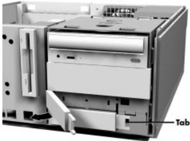
*Removing the blank panel*
