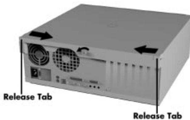
*Loosening the screw and pressing the tabs*
