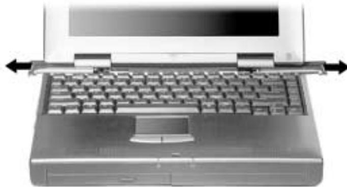
4. Gently lift up the edge of the keyboard nearest the LCD and slide the keyboard toward the LCD screen to release the tabs that secure it.
