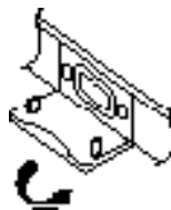
Opening the serial port cover
