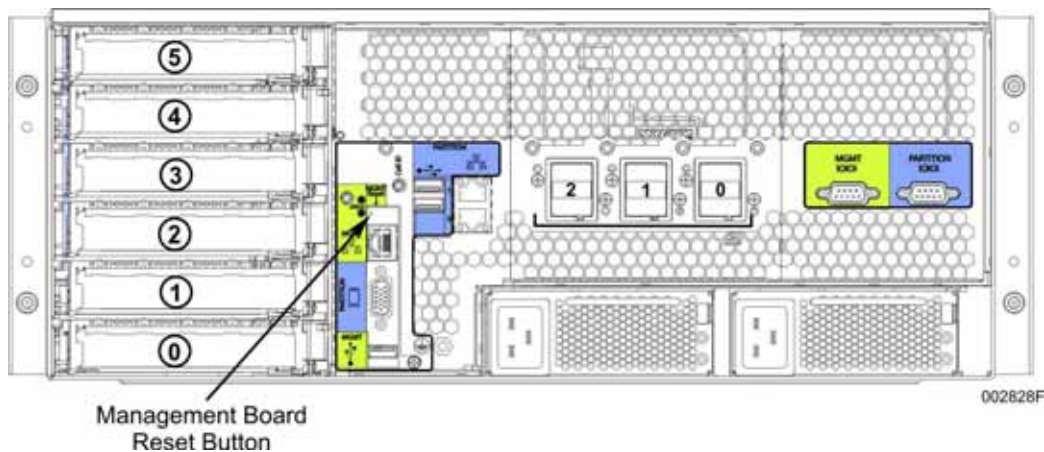
Figure 3-3 Location of Management Board Reset Button
