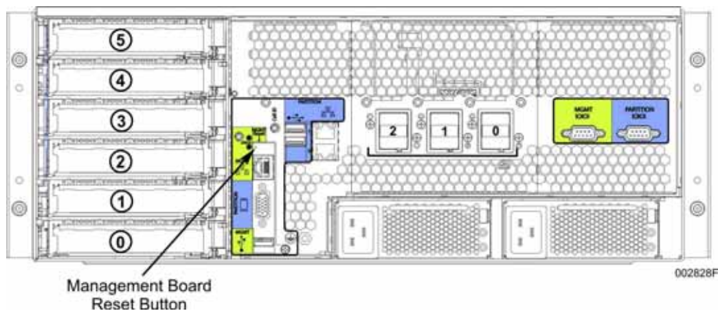
Figure 3-4 Location of Management Board Reset Button
