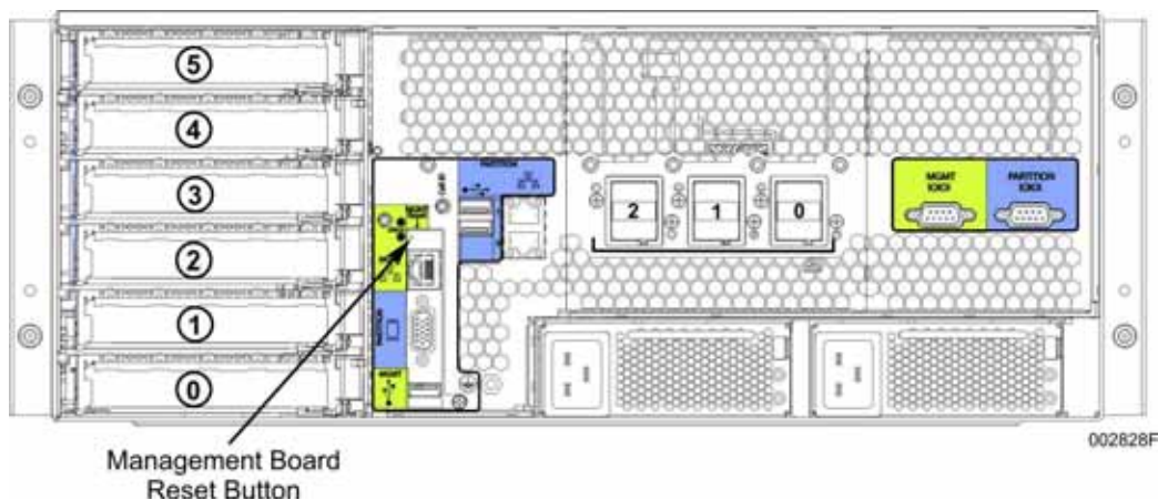
Figure 3-5 Location of Management Board Reset Button
