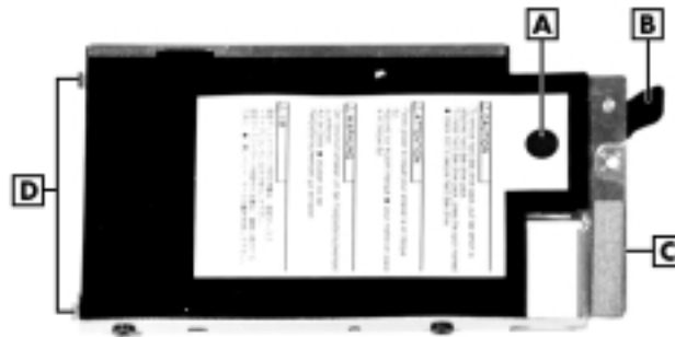
A – Black Dot B – Hard Disk Drive Tab C – Drive Bracket D – Metal Tabs
